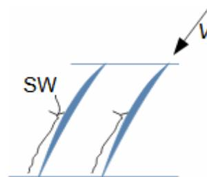
18: Formation of a  $\lambda$ -shock wave in compressor profile cascade
