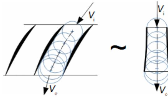
17: Geometric similarity of diffuser blade cascade with symmetrical diffuser
