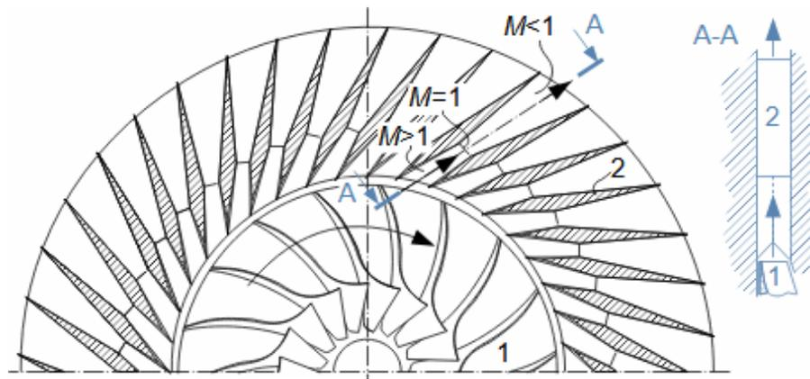
19: Example of supersonic turbocompressor arrangement
