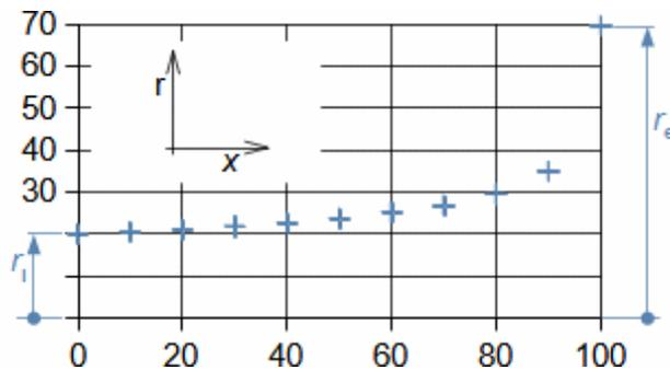
Calculated radius of diffuser with constant pressure gradient - so-called cornut shape [Frass, 1989, p. 156].  $r$  [mm];  $x$  [mm].
