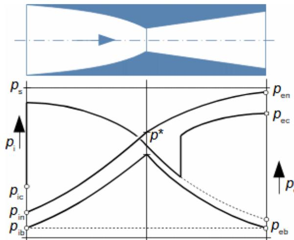
16: Effect of inlet velocity change on supersonic diffuser function
