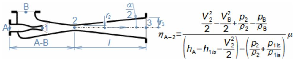
$$\eta_{A-2} = \frac{\frac{V_2^2}{2} - \frac{V_B^2}{2} + \frac{p_2}{\rho_2} - \frac{p_B}{\rho_B}}{\left(h_A - h_{1is} - \frac{V_2^2}{2}\right) - \left(\frac{p_2}{\rho_2} + \frac{p_{1is}}{\rho_{1is}}\right)} \mu$$
