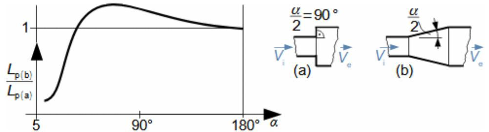
**12:** Effect of cone diffuser angle on pressure drop
