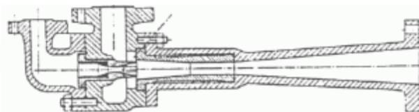
**22:** Example of steam ejector in function as a steam condenser vacuum cleaner [Nožička, 2000]
