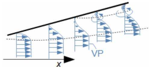
10: Mechanism of boundary layer separation from diffuser wall and subsequent vortex formation
